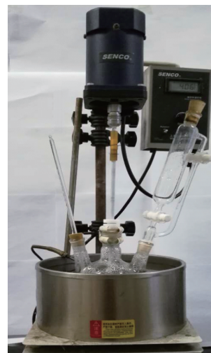
Fig 2 Photograph of experimental device for preparing \text{Fe}_3\text{O}_4 nanoparticles
